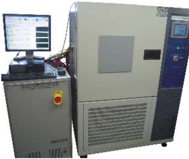
[電流源+温度制御部]
